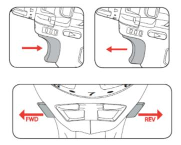
The drill is turned ON and OFF by pulling and releasing the trigger switch
