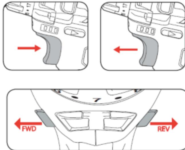
The drill is turned ON and OFF by pulling and releasing the trigger switch
