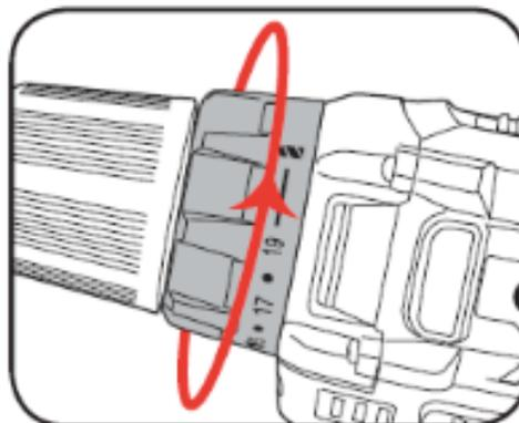
This tool is fitted with a torque adjustment ring to select the operating mode and to set the torque for tightening screws. Large screws and hard workpiece materials require a higher torque setting than small screws and soft workpiece materials.
